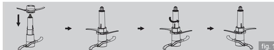
4. Install the blade to the spindle (fig. 2).
